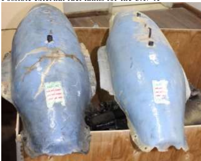
Figure 12.6 Possible external fuel tanks for the UAV-X
