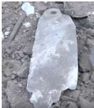
Figure 33.G.1 Rear wing of Paveway guidance unit
