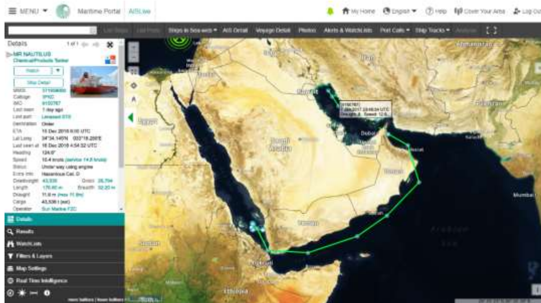
Figure 21.13 AIS track of MR Nautilus from 1 December 2016 to 10 March 2017 (Iran - Ras Issa, Yemen)
