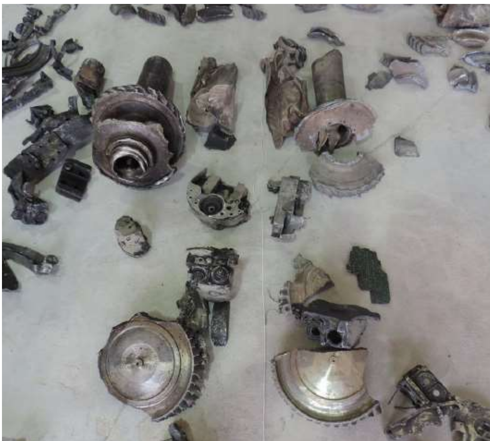
Figure 11.4 Significant debris of the two Microturbos with characteristics similar to TRI-60-2
