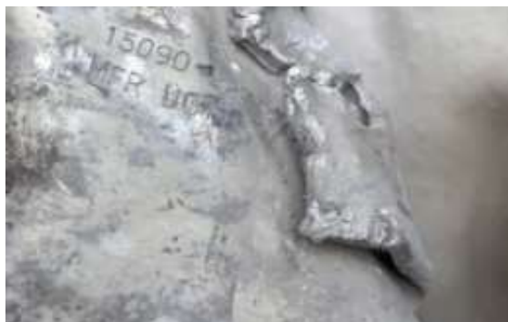
Figure 33.G.3 Fragmentation from Paveway guidance unit
