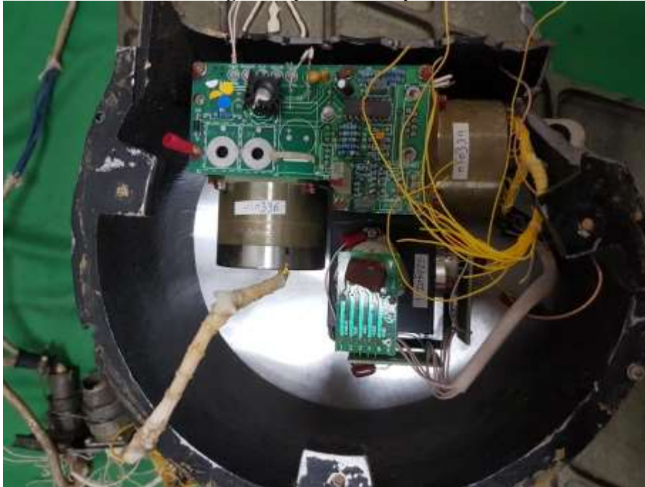
Figure 13.1 Debris of the inertial navigation system on its platform
